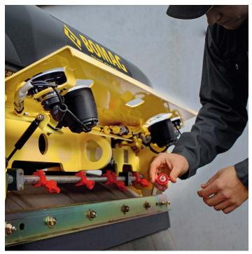
When the spray tips themselves need cleaning, remove the tips from the spray bar and use a welding tip cleaner to get into the crevices. Photo courtesy of BOMAG Americas
