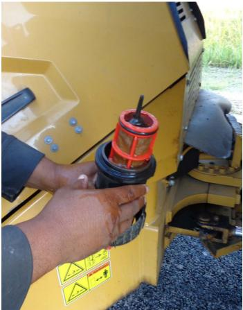
Use a toothbrush dipped in chlorine-and-water solution to scrub the filter screens clean before rinsing the filter with clear water and reassembling the filter. Double-check the O-ring to ensure it's free of damage before replacing the filter in the tank. Photos courtesy of John Ball of Top Quality Paving & Training
