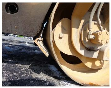
If the spring is damaged, it can't hold the scraper bar in place properly. Check this on your daily walk-around and make sure it gets fixed. Photo courtesy of John Ball of Top Quality Paving & Training
