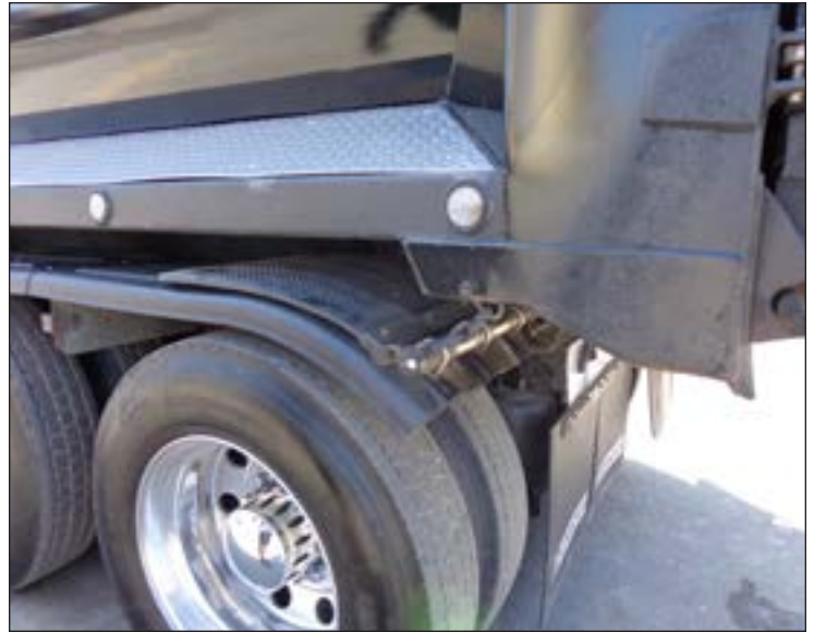
LEFT: These four mud flaps end in a sensible row. Steve Murray of Steve Murray Trucking, Hooksett, New Hampshire, uses four flaps to completely shield motorists behind his truck. Notice the flaps on the left and right hang from chains of seven links each. RIGHT: The chain is long and flexible enough to allow Murray to lay the mud flap on the fender where it doesn't touch the push roller of the paver. This allows good contact between the push roller and truck tire. It also protects the mud flap from tearing or from getting caked with asphalt.
