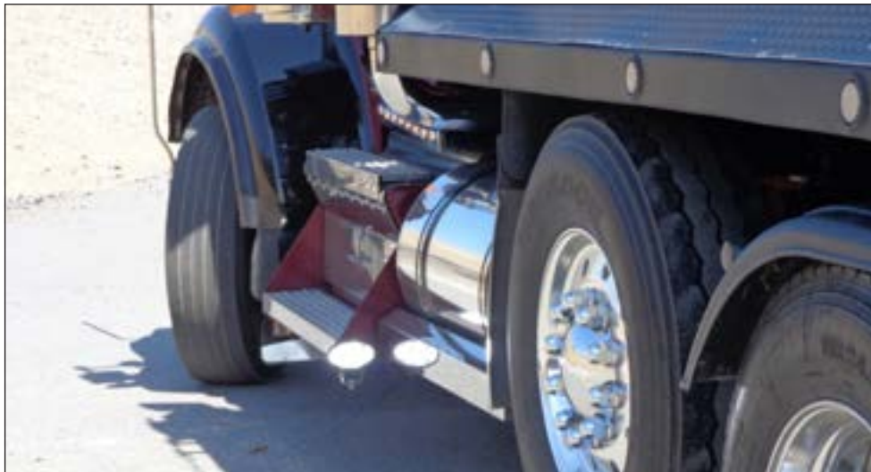
The placement of this oval-shaped LED allows it to shine toward the paver, illuminating the wheels and the area where the paver's push roller will come in contact with the back tire. The driver wants to see that there is nothing between his vehicle and the paver as he's backing.
