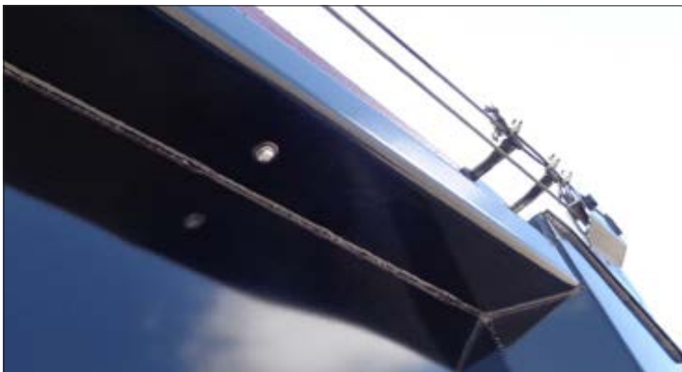
Murray's truck has LEDs installed so that they shine down from the tarp/canopy track; this illuminates and outlines the side of the truck.
