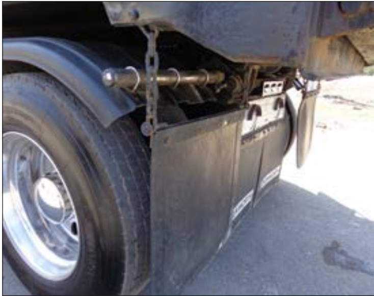
LEFT: These four mud flaps end in a sensible row. Steve Murray of Steve Murray Trucking, Hooksett, New Hampshire, uses four flaps to completely shield motorists behind his truck. Notice the flaps on the left and right hang from chains of seven links each. RIGHT: The chain is long and flexible enough to allow Murray to lay the mud flap on the fender where it doesn't touch the push roller of the paver. This allows good contact between the push roller and truck tire. It also protects the mud flap from tearing or from getting caked with asphalt.
