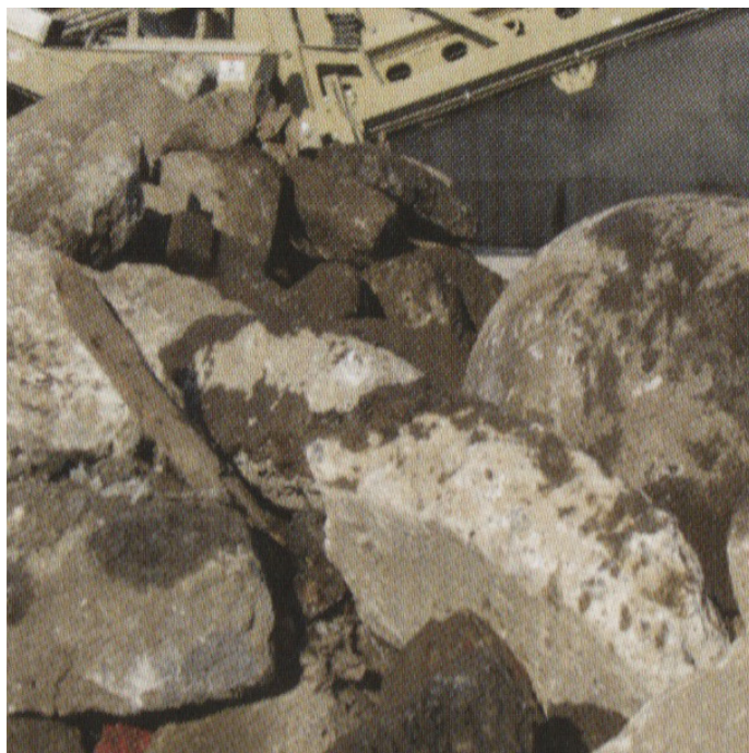
Recycled material (above on left) is ready to be processed. After it's processed through an FT4240 impact crusher, it's a more uniform size (above on right).
