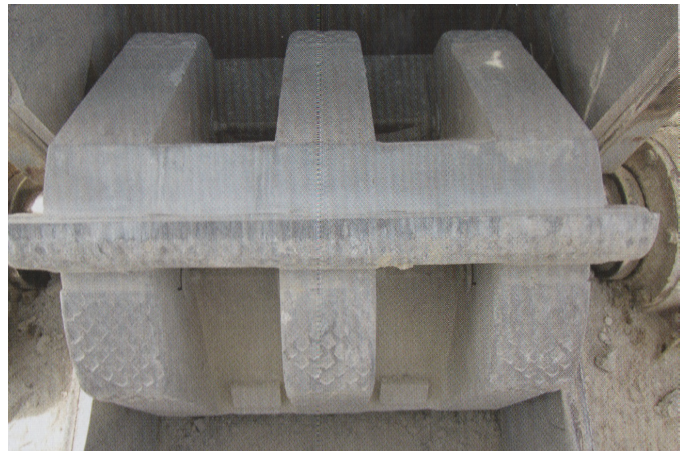
This blow bar shows minimal wear; it's not quite ready for replacement.
